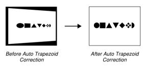
Note that auto trapezoid correction must be turned on to be performed. In addition to correcting rectangular shapes, auto trapezoid correction also sharpens text outlines and brightens the background of the image, making its contents easier to view.
